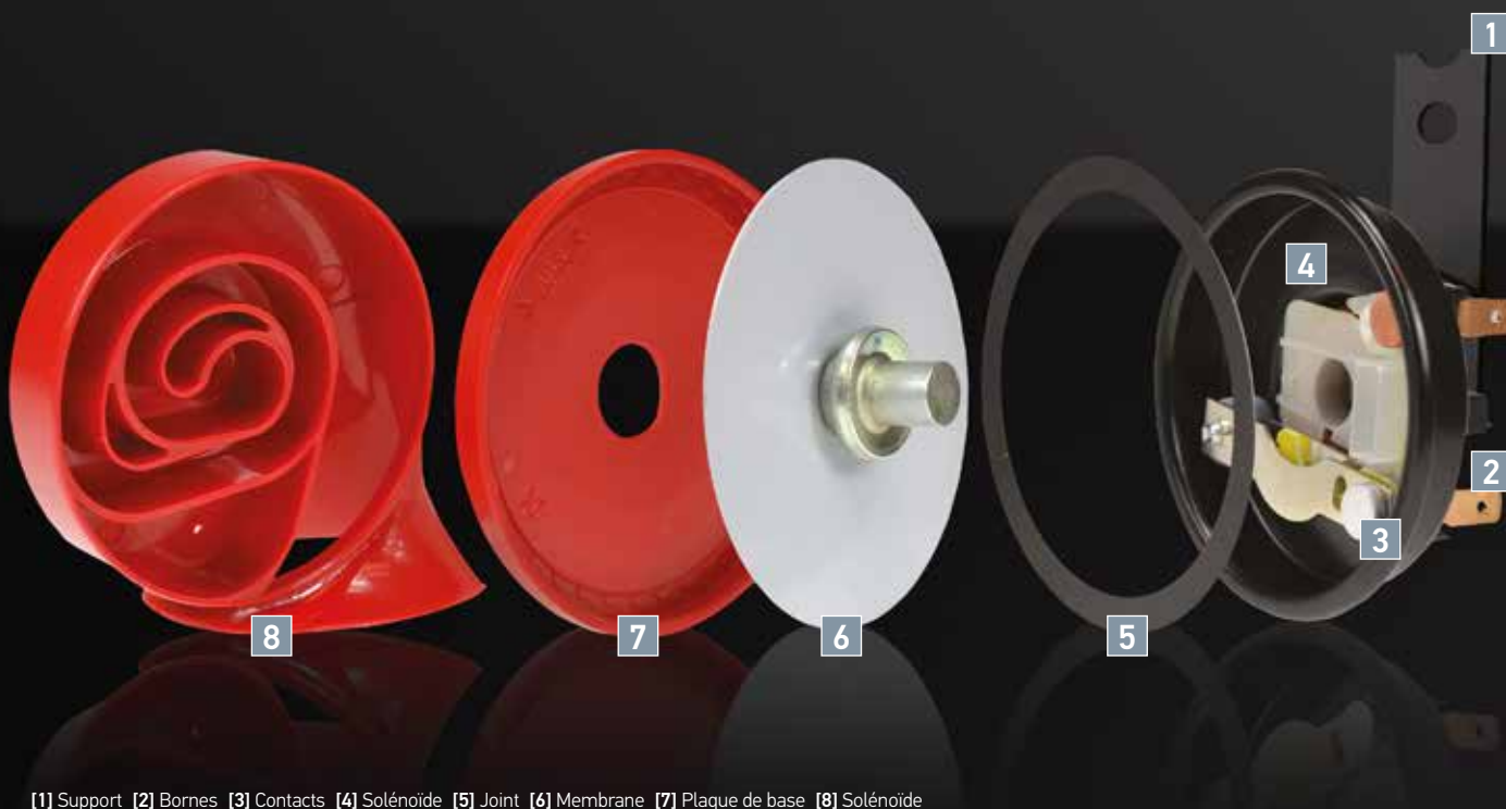
[1] Support [2] Bornes [3] Contacts [4] Solénoïde [5] Joint [6] Membrane [7] Plaque de base [8] Solénoïde
