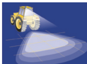
High installation position Fig. 3
