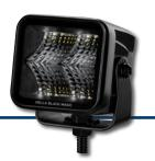
Upright or pendant surface mounting, multi-voltage 10-30 V, power consumption 20 W, light output 1,400 lm, degree of protection IP 68/IP 69K, ECE type approval: ECE R10, connection 500 mm cable with DEUTSCH DT connection
