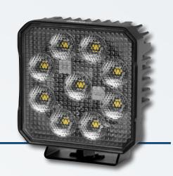
Upright or pendant surface mounting, multi-voltage 10 - 30 V, 9 LEDs, power consumption 31 W, light output 3,000 lm, degree of protection IP 6K7/IP 6K9K, ECE R10 approval, 800 mm cable connection, thermal management system\*\*
