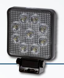
Upright or pendant surface mounting, multi-voltage 10 - 30 V, 9 LEDs, power consumption 9 W, light output 1,000 lm, degree of protection IP 6K7/IP 6K9K, ECE R10 approval, 800 mm cable connection
