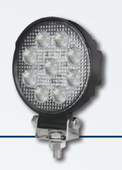
Upright or pendant surface mounting, multi-voltage 10 - 30 V, 9 LEDs, power consumption 15 W, light output 1,500 lm, degree of protection IP 6K9K, ECE R10 approval, connection 800 mm cable
