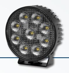
Upright or pendant surface mounting, multi-voltage 10 - 30 V, 9 LEDs, power consumption 31 W, light output 3,000 lm, degree of protection IP 6K7/IP 6K9K, ECE R10 approval, 800 mm cable connection, thermal management system\*\*
